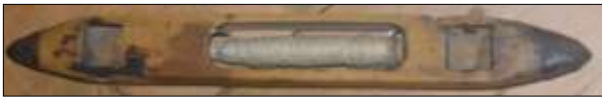
The flying shuttle, invented by John Kay (1733, France) significantly speeded up the weaving process thereafter.
